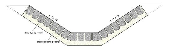
Figure 3: Cross-sectional profile of a ditch with basic technical parameters (source: VÚV TGM, v.v.i.)
