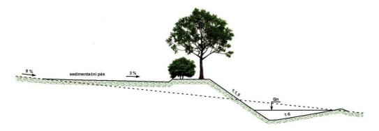
Figure 11: Schemata of basic technical parameters of a baulk in the slope profile (source: VÚV TGM, v.v.i.)
