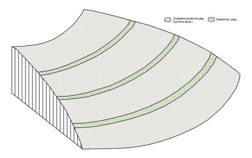
Figure 5: Schematic of an infiltration belt with a longitudinal slope profile (source: VÚV TGM, v.v.i.).
