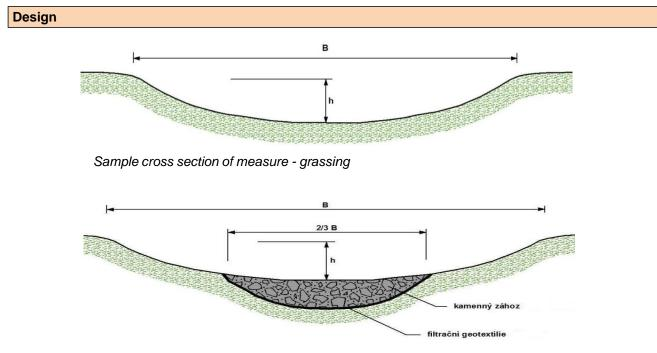
Sample cross section of measure - backfill
