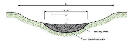
Figure 7: Cross-sectional profile of a stabilization pathway with basic technical parameters (source: VUV TGM, v.v.i.).
