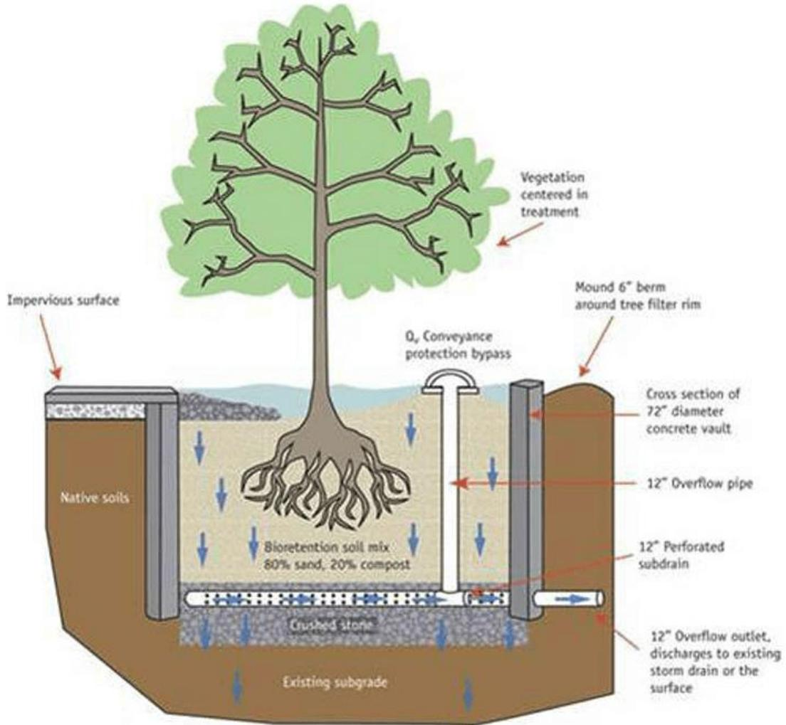
Figure: 39. Stormwater tree trench (<https://mediaborough.blog/2018/05/17/stormwater-projects-in-the-borough/#jp-carousel-108>)
